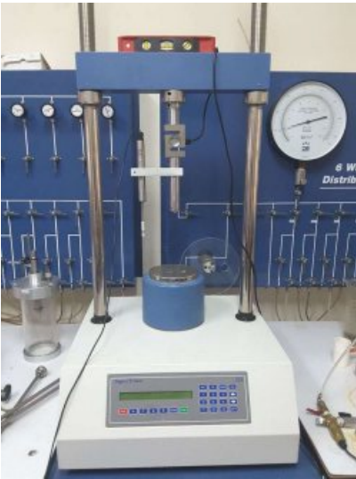
Figure C-5 Unconfined compression test apparatus
