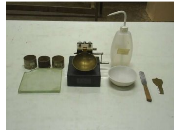
Figure C-3 Liquid limit and plastic limit test devices
